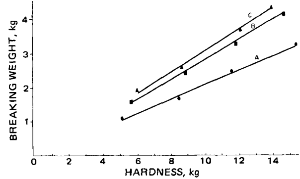
Figure 7 —Effects of tablet concavity on the mechanical strength of a 7.035-mm wide × 17.900-mm long × 6.350-mm thick lactose capsule-shaped tablet. Key: A, 1.143 mm deep; B, 1.8034 mm deep; and C, 2.235 mm deep.
